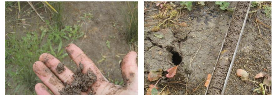
Fig.6 Soil sample and ribbon test showing soil breaking up, indicating low clay content
