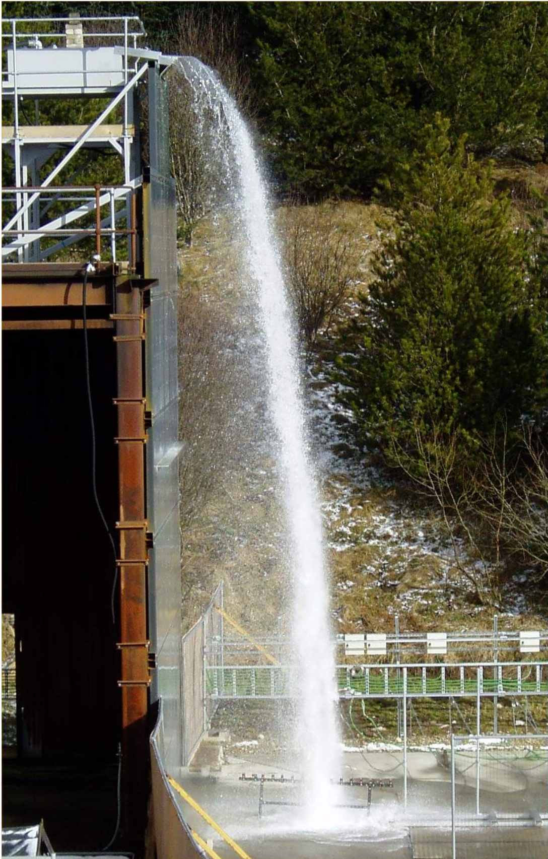
Figure 15: Development of a free cascade (21 kg/s). A diffuse spray separates from the inner edge of the cascade and falls between the main flow and the tank wall.
