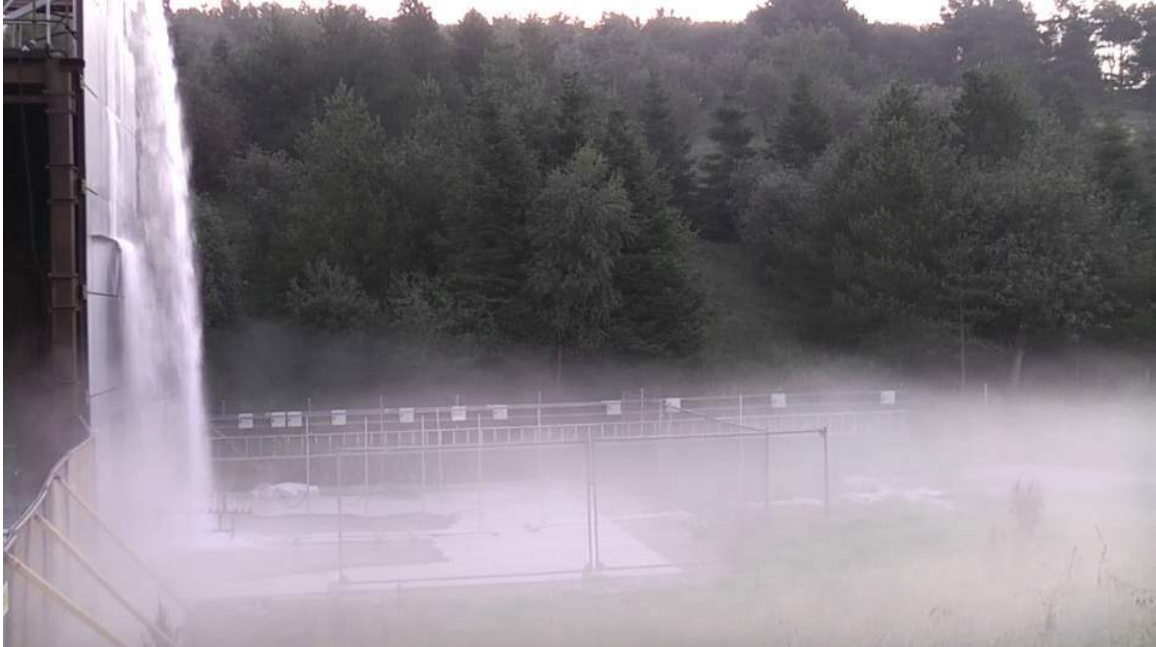
Figure 33: Cascade structure and vapour cloud formation during Test 13 (15 kg/s hexane).
