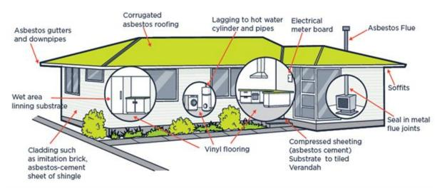
Stringent procedures must be followed if asbestos is discovered during construction. Work methods, equipment and safety procedures must be in accordance with the New Zealand Guidelines for the Management and Removal of Asbestos.
