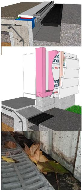
Acceptable Solution E2/AS1 permits the use of channel drains across door openings for **provision of level access only**. Where building consent applications utilise this acceptable solution design plans **must** include **design detailing** showing clearance of wall cladding and wall framing, adjacent the door opening, in relation to finished ground and channel drain ends.
